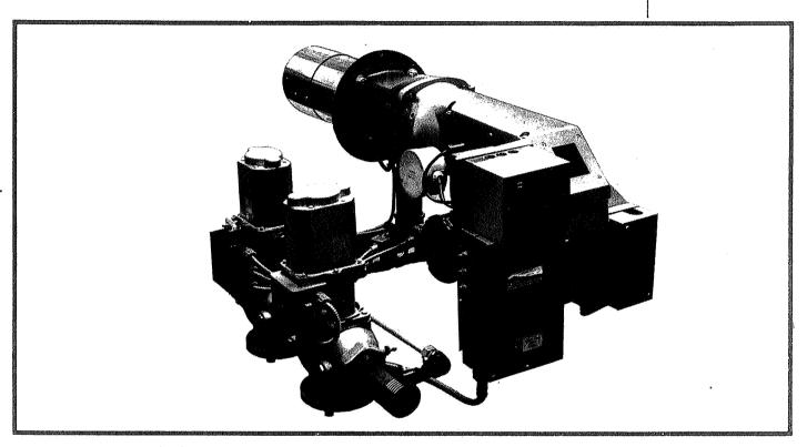
The Nu-Way model CG4/24 blown gas burner is marketed to meet the requirements of international markets and has rated outputs in the range 146-454 kW (125000 - 387500 kcal/h: 500,000 - 1,550,000 Btu/h). Built to comply with relevant standards, the burner will fire pressurised systems having resistances as listed under burner selection. Units are available for both on/off and high/low/off operation.
