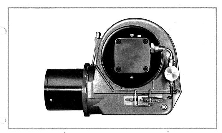
The Nu-way C2 pressure jet burner is designed for automatic operation with burner outputs from 187 000 625 000 Btu/h (55–182 kW, 47 500–157 000 kcal/h) against balanced draught conditions. Available for on/off operation only.
